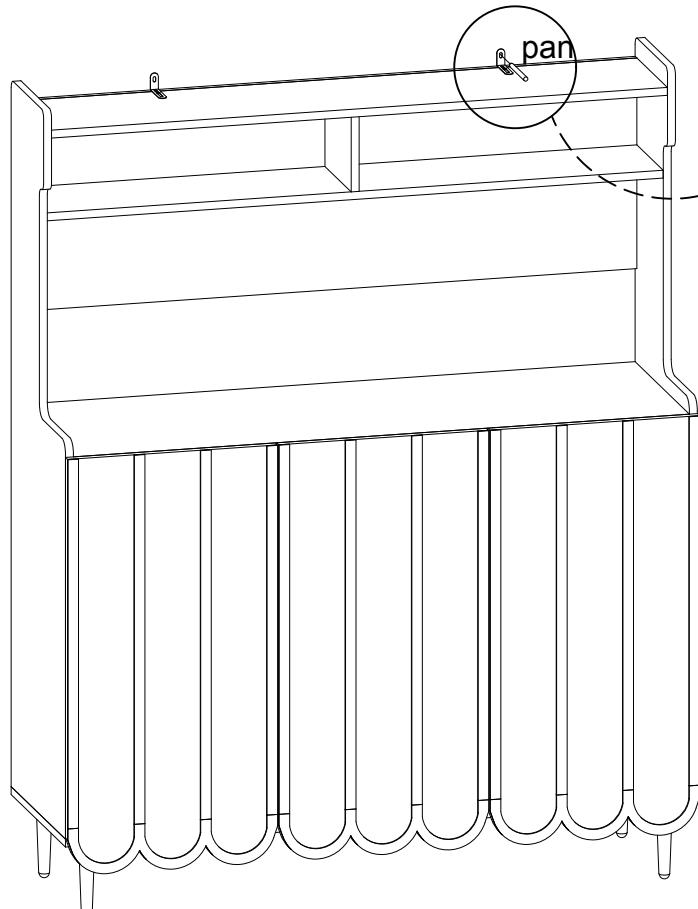
To prevent children from climbing and dumping parts, first move the cabinet to the wall, then use pen to make hole in the wall of O parts, remove the cabinet and punch holes in the marked position with M6 drill, then punch L into the hole, then move the cabinet to its original position and secure it with Screw M.
