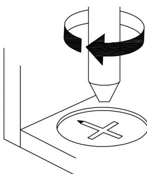
**EN**\_Turn cam lock clockwise to tighten.
