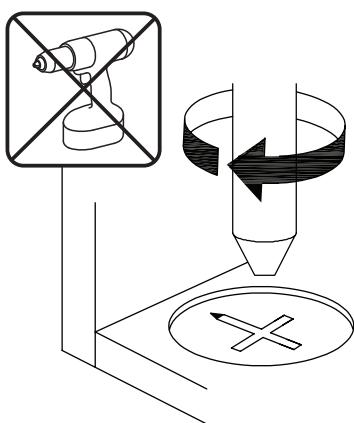
**EN** Turn cam lock clockwise to tighten.
