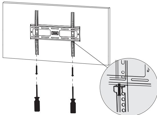
Hook the TV to the wall plate, For additonal Security, tighten the screws(a). Tighten or loosen the screw(b) to make the tilt happen.
