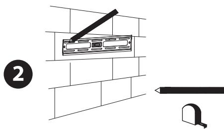
Draw the mounting holes with a pen, and use the tool(H) to make sure in level.
