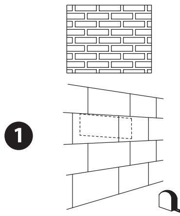
Find a reasonable position for mounting. Please do not drill in masonry joints!
