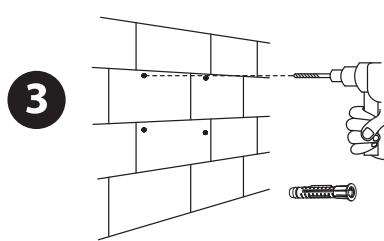
Drill holes with a 10mm Stone drill, use Concrete Anchor(D)
