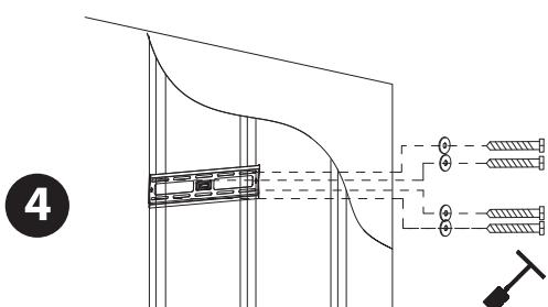
Attach the Part A to the wall using the supplied screws or your own suitable screws, there are long holes to adjust the holder perfectly.
