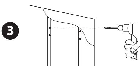
Drill holes with a 4.5mm wood drill.
