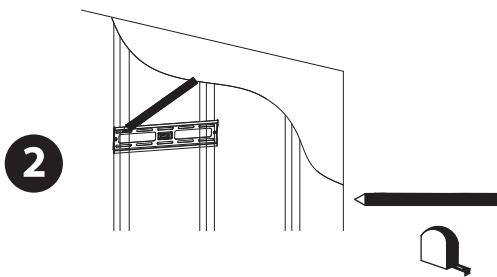
Draw the mounting holes with a pen, and use the tool(H) to make sure in level.
