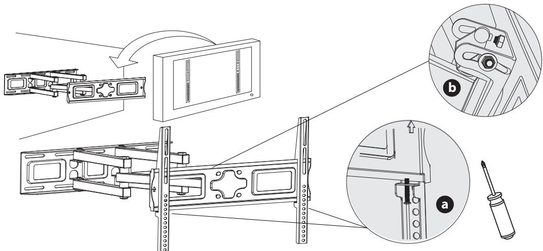
Hook the TV to the wall plate, For additonal Security, tighten the screws(a). Tighten or loosen the screw(b) to make the tilt happen.
