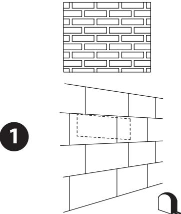
Find a reasonable position for mounting. Please do not drill in masonry joints!
