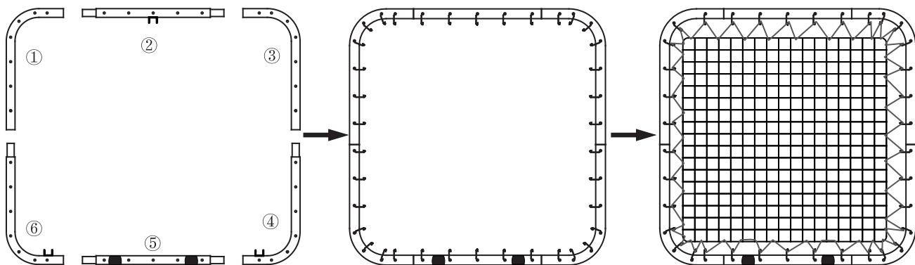
**EN** Hang the elastic cords on the hooks starting with the ones on the four corners, and then hang the remaining elastic cords one by one.
